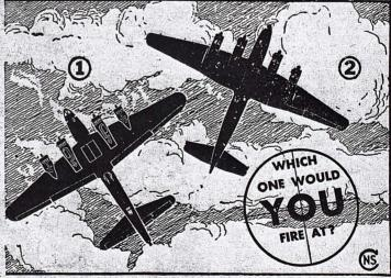
NOT AT NO. 1! It's the AAF's famous B-17 Flying Fortress, a low-wing heavy bomber powered with four radial engines. The nose of the long, streamand the tail extends beyond the tailplane. Both edges of the President Roosevelt revealed wings taper evenly to rounded tips. The tailplane has tapered edges, rounded tips and a single
