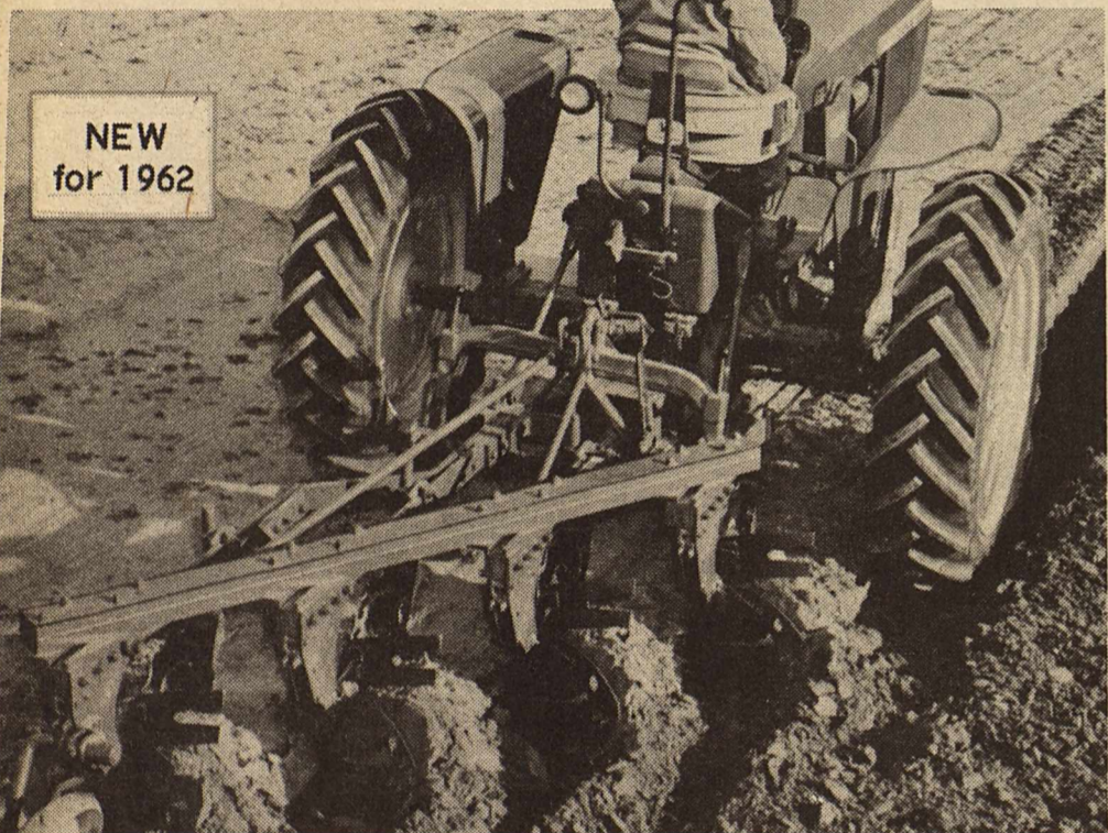
Line-of-draft hitching and a wide range of easily made, precise adjustments are among many reasons why John Deere Plows do such good work.
