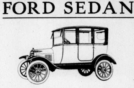
Five Passenger-Four Cylinder-and Twenty Horse-Power. Large sliding plate glass windows in doors and the sides. Roomy Doors. Two unit electric starting and lighting system. Demountable rims, 8 1-2-inch Non-skid tires all round. Tire carrier. An all season car of style and comfort-for social functions, for shopping, for touring and general uses. Enclosed car comforts with Ford simplicity and reliability.
