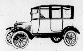
Five Passenger—Four Cylinder—and Twenty Horse-Power. Large sliding plate glass windows in doors and the sides. Roomy Doors. Two unit electric starting and lighting system. Demountable rims, 3 1-2-inch Non-skid tires all round. Tire carrier. An all season car of style and comfort-for social functions, for shopping, for touring and general uses. Enclosed car comforts with Ford simplicity and reliability.
