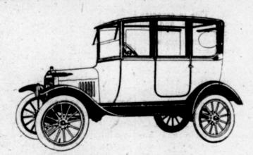
Five Passenger-Four Cylinder-and Twenty Horse-Power. Large sliding plate glass windows in doors and the sides. Roomy Doors. Two unit electric starting and lighting system. Demountable rims, 3 1-2-inch Non-skid tires all round. Tire carrier. An all season car of style and comfort-for social functions, for shopping, for touring and general uses. Enclosed car comforts with Ford simplicity and reliability.
