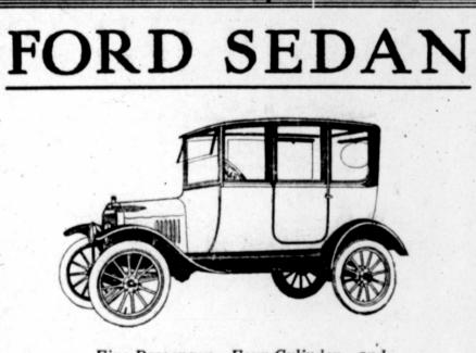
Five Passenger-Four Cylinder-and Twenty Horse-Power. Large sliding plate glass windows in doors and the sides. Roomy Doors. Two unit electric starting and lighting system. Demountable rims, 3 1-2-inch Non-skid tires all round. Tire carrier. An all season car of style and comfort-for social functions, for shopping, for touring and general uses. Enclosed car comforts with Ford simplicity and reliability.
