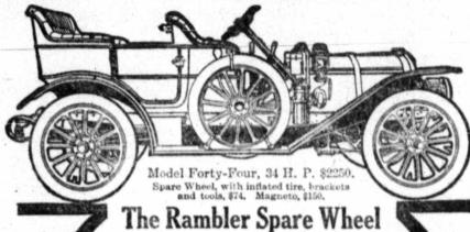
All the new four-cylinder Ramblers are fitted for the Rambler Spare Wheel-a wheel complete-excepting the hub center, on which is carried a complete tire inflated. The regular wheel is secured to the hub center by Removing the six nuts for these bolts this wheel can be detached in two minutes with the special tools provided and the Spare Wheel put on and secured in three minutes.
