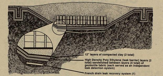
CONSTRUCTION AND OPERATION -- The trench will be constructed approximately 20 feet deep, 200 feet wide and 2,200 feet long. A host of environmental safeguards will be incorporated including five independent barriers against leaks, four independent leak detection systems, and one leak recovery system. In addition, the pit will be ringed with a series of monitor wells. Yet, NO LIQUIDS WILL BE BURIED in the facility.
