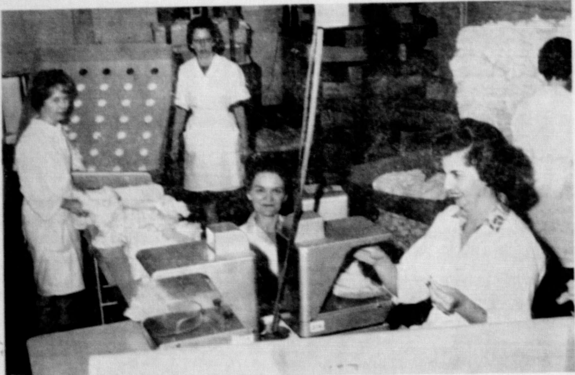
SECOND CREW —Shown above is the second micronaire crew of the classing office. The samples are brought from the storeroom to the micronaire room. The crew, (left to right) Jerrie Nabers, Alyene Sims and Beverly Philpot, handle the weighing, micronaireing and stacking of samples. Deane Bradshaw, supervisor, is shown in the background. Both crews handle about 4,000 samples daily.
