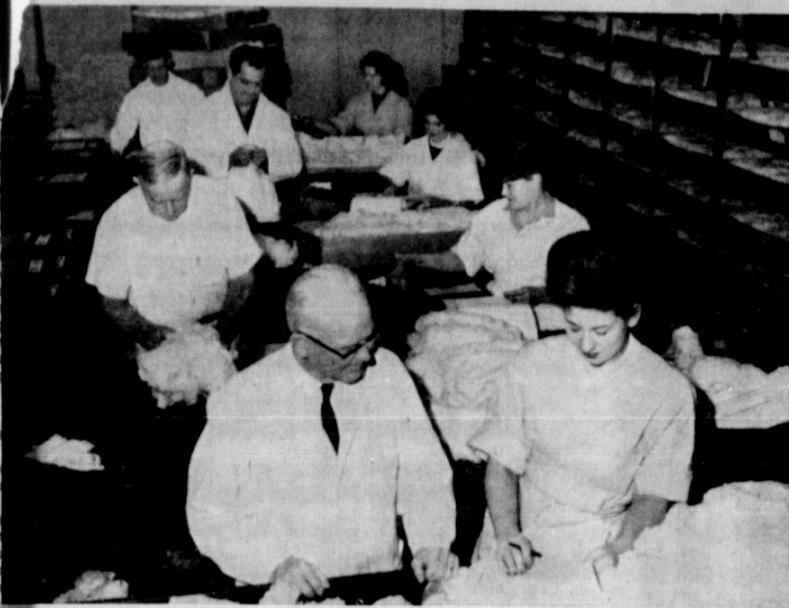
CLASSING —The heart of the cotton classing operation is the classing room, a special conditioning room, always maintained at 71 degrees and the desired air density. Samples are brought to the room in trays where they stay until conditioned. The classers determine grade and staple and recorders make proper notations. From front to back are: John Egan and Betty Evans, Milton Hall and Marilyn Whitten, Frank Ortiz and Brenda Egan and Shirley Sewell and Teresa Miller. The samples are then put on a conveyor belt bagged, as property of the U. S. Government.
