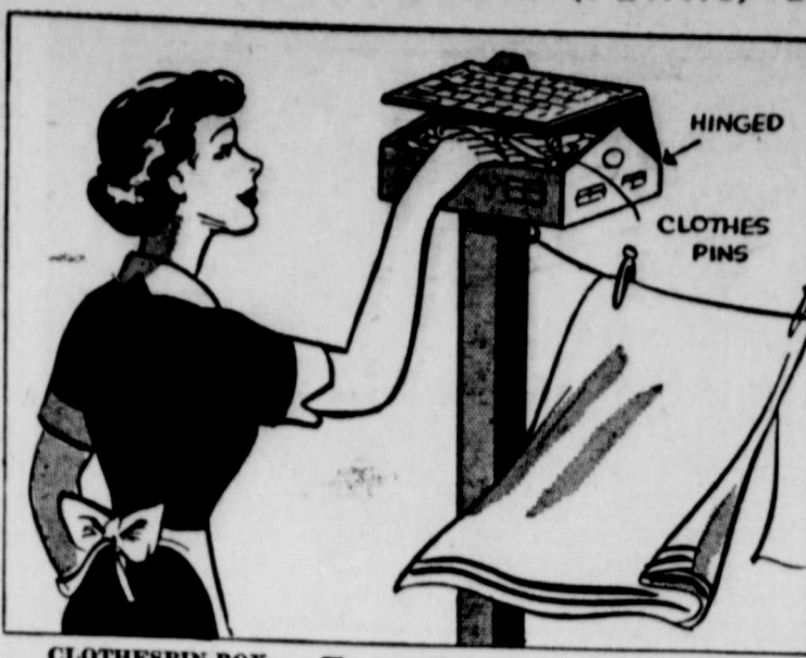
CLOTHESPIN BOX . . . The man of the house, if handy with tools, can make the above clothespin box without difficulty. It can be made of scrap wood and mounted at a handy spot. The hinged roof makes the pins accessible.
