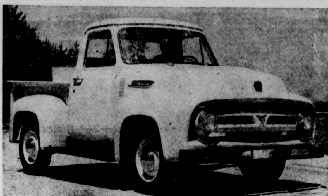
TRANSMISSION FIRST—The new 1953 Ford F-100 series of pick-up and panel delivery trucks will be available for the first time with fully automatic Fordomatic transmission. It also can be had with four other transmissions, including automatic overdrive. The F-100 features an entirely new "driverized" cab, a new one-piece, curved windshield and a 4-foot wide rear window.
