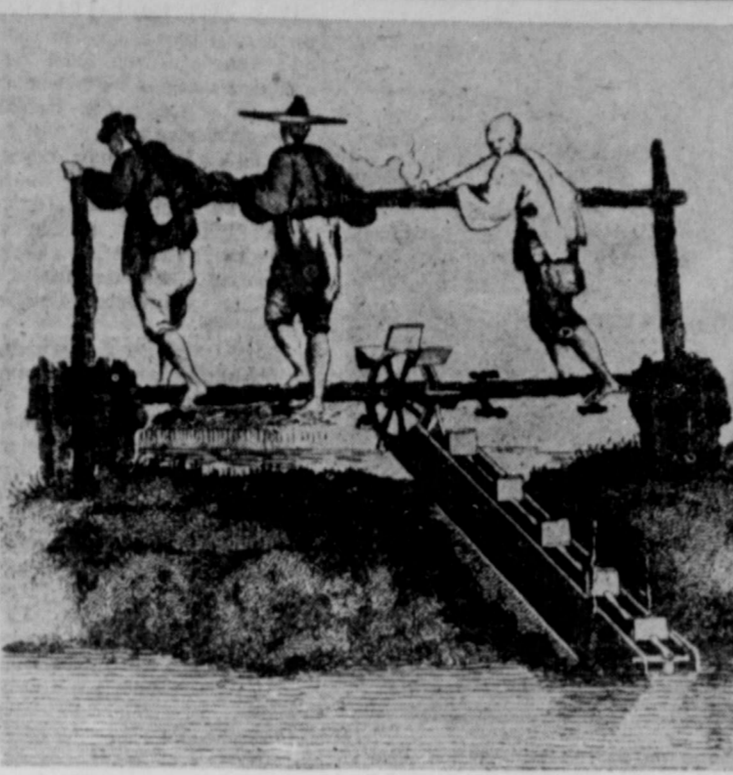
A Chinese dragon wheel was used for pumping water in the third century before the Christian era when China first realized the need for irrigation. In that century, Li Ping, a territorial governor, planned a great dike with a series of channels, ditches and barriers which would divert the Min-Ho river and send its water over the parched fields. Today's dams, power pumps, canals and underground mains accomplish with greater efficiency the same purpose which the Chinese held, to avoid complete depe deace upon natural rainfall.
