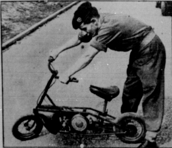
Motor scooters are now part of the gun-knife-grenade equipment of Allied paratroopers. The collapsible little vehicles can scoot a chutist along at 40 to 45 m.p.h. for 100 miles on one gallon of gasoline.
