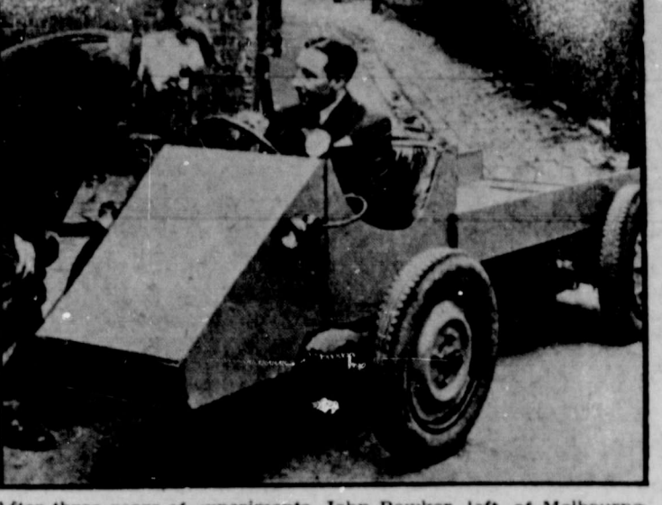
After three years of experiments, John Bowker, left, of Melbourne, Australia, comes out with this solution to the transportation problem. The electric vehicle can go 30 m.p.h., has run continuously for 111 miles. A battery recharge costs 50 cents. Len, John's brother, sits in the seat.
