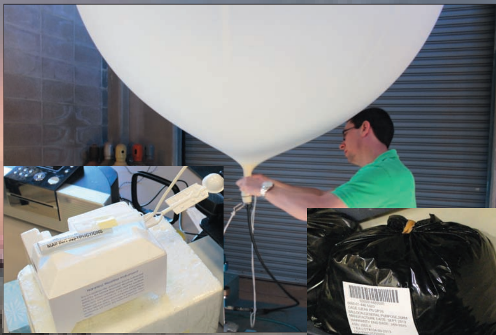
Justyn Jackson assembles a weather balloon as a demonstration for The Pampa News. Left, the instruments that are attached to the weather balloon, which measure wind speed, humidity and other weather conditions. It also has a GPS system installed for tracking. Right, the package the balloon comes in.
