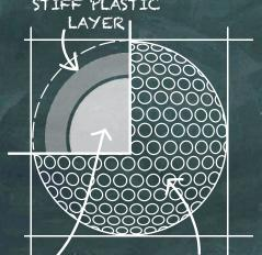
HIGH FRICTION SOLID, RUBBER COVER BOUNCY RUBBER CORE
