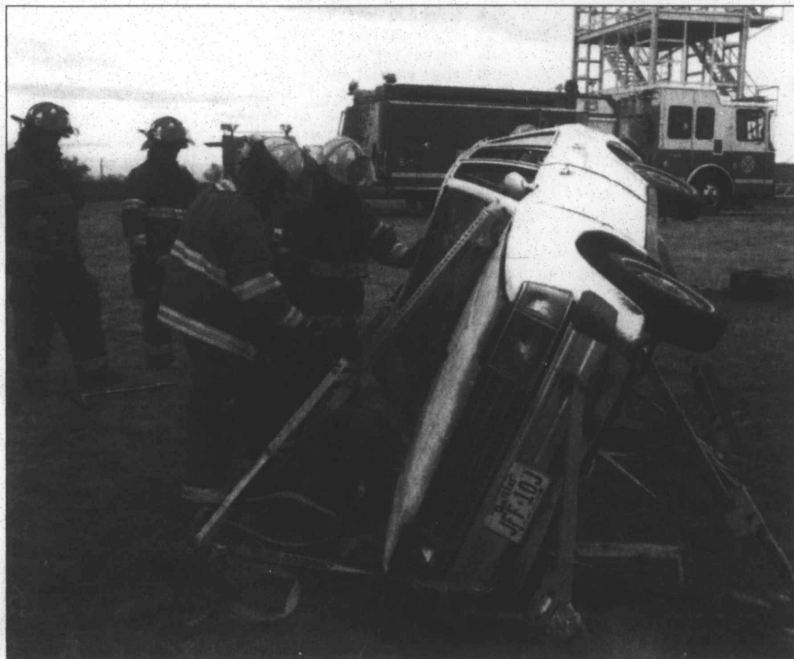
staff photo by Betsy Phillips Pampa Fire department personnel participate in ongoing training with vehicle stabilization equipment purchased by the department last fall. The equipment, known as Res-Q-Jack, compliments the department's state-of-the-art TNT extrication equipment, Capt. Keith Arnzen, Capt. Jesse Hanes, (foreground) Firefighter Travis Dosch, and Equipment Operator Jim Sirmans.
