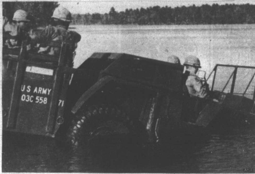
WASH DAY—Soldiers of the 82d Airborne Division, Ft. Bragg, N.C., test one of their 550 newly-acquired Gamma Goats—the Army's replacement for the M37 3/4-ton truck. Designated the M561, the Gamma Goat provides improved mobility for forward area units engaged in operations over a variety of land and water obstacles.
