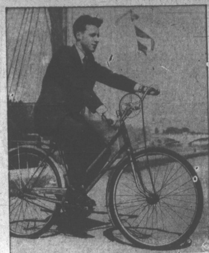
HANDY CYCLE —French inventor Charles Duval, above, thinks he's solved a big problem for cyclists. He claims that leg-muscle strain can be eased by switching to hand pedals which he has mounted on his bike's handlebars. Or, if you prefer to make like a jet, you can use both hand and foot pedals to increase your speed. The gadget is one of many shown at the annual inventors' exhibit in Paris.
