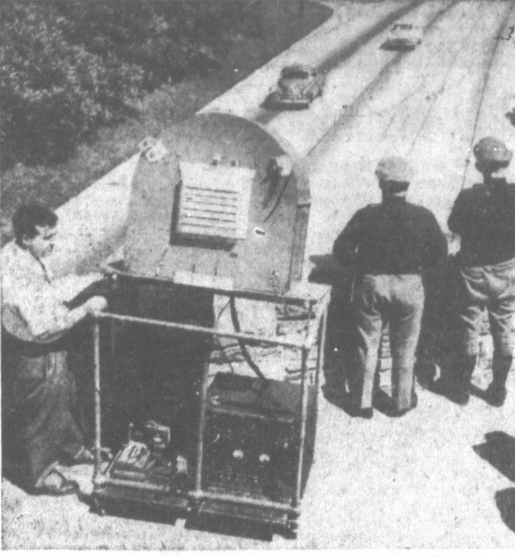
RADAR EYE ON SPEEDERS —Parkway police in Westchester County, N. Y., try out a new radar camera in clocking speeding autos. When a car exceeding the speed limit enters the radar beam, an electric switch is tripped and the camera takes a picture of the speeding car on 16-mm. movie film. A case is being prepared to test the device's legality in court cases.
