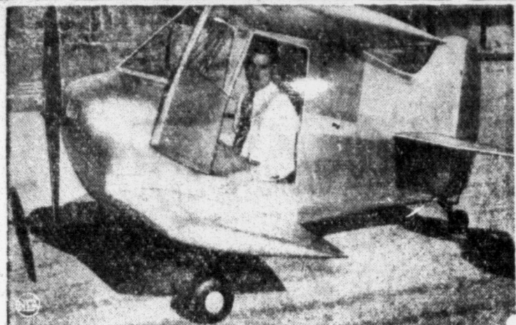
"DRESSED" IN A PLANE—"I feel like I was wearing her instead of flying her," said Test Pilot Bob Starr after taking up "Sky Baby" the world's smallest plane on its first flight at Palm Springs, Calif. The midget has a wingspread of only seven feet, three inches, is nine feet 10 inches long, weighs 452 pounds and is powered by an 180-pound, 85-h.p. Continental engine that turns a 60-inch wood-and-plastic propeller. Starr, shown in the plane, and Ray Stitt, of Riverside, Calif., built Sky Baby for about $2200.
