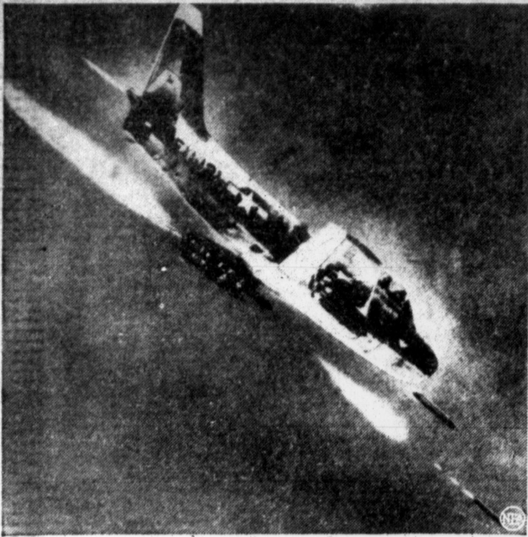
ROCKET PRACTICE —North American F-86 Sabre Jet tests its five-inch rockets on the gunnery range near Nellis Air Force Base, Nevada. Carried in clusters under each wing, the rockets can be fired singly or in salvos. Rockets like these are in use in Korea.
