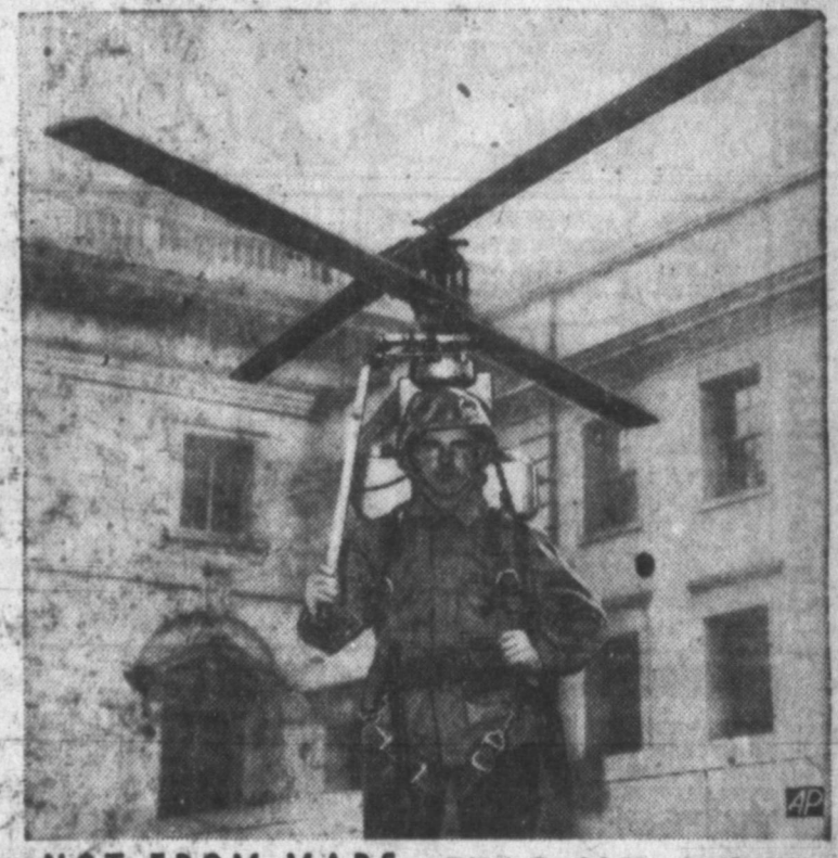
NOT FROM MARS —T/Sgt. Daniel Murphy demonstrates "Hoppi-Copter," a one-man helicopter strapped to shoulders and capable of flying a fully-armed man, in Washington, D. C.
