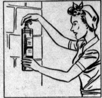
Grasp handle of vaporizing liquid (pump gun) extinguisher and pull toward you to remove from bracket.
