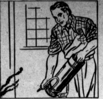
Keep a firm grip on the nozzle, as you turn the soda acid or foam extinguisher over to operate it.
