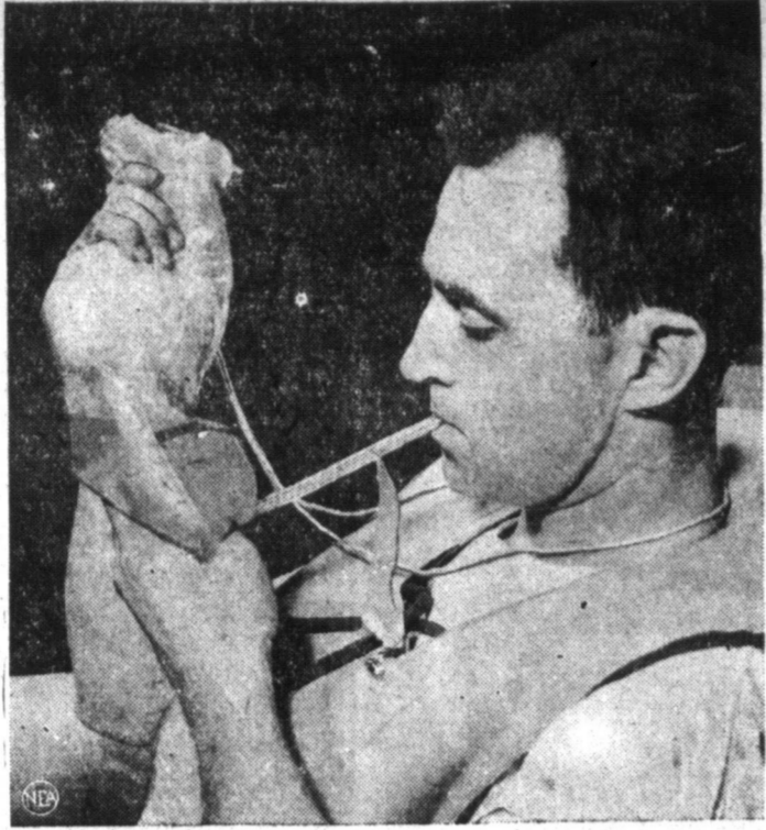
Purifying device demonstrated here by sailor converts salt water into drinking water—a boon to seamen and flyers adrift at sea. Water is put in top part of bag and squeezed through chemicals that filter it. All life rafts will carry this equipment.
