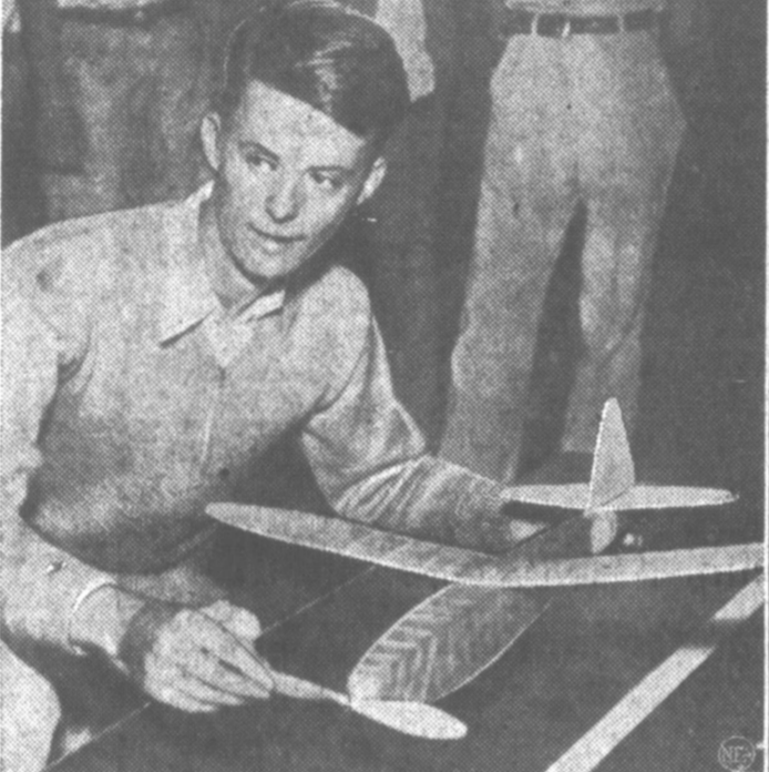
This trim yellow model plane, flashing over an 88-foot course in one second, set a world speed record of 60 miles an hour for model aircraft. Its owner, Leonard Becker, 18, Lakewood, O., is shown with his speedster just before the takeoff in the Scripps-Howard junior aviator national air races in Cleveland, O. The plane is powered with a rubber band motor and during part of its flight, watched by a great crowd, traveled several miles faster than its 60-mile average.
