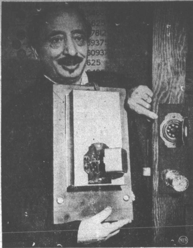
Edmond Michel, of Chicago, shows his new keyless door lock which can be set to any of 764 combinations. Absent householder, upon return, pushes proper buttons on dial seen at right and door opens. Lock can be set in connection with an alarm so that puffing wrong buttons rings a loud bell, or device can be hooked up with telephone alarm system.
