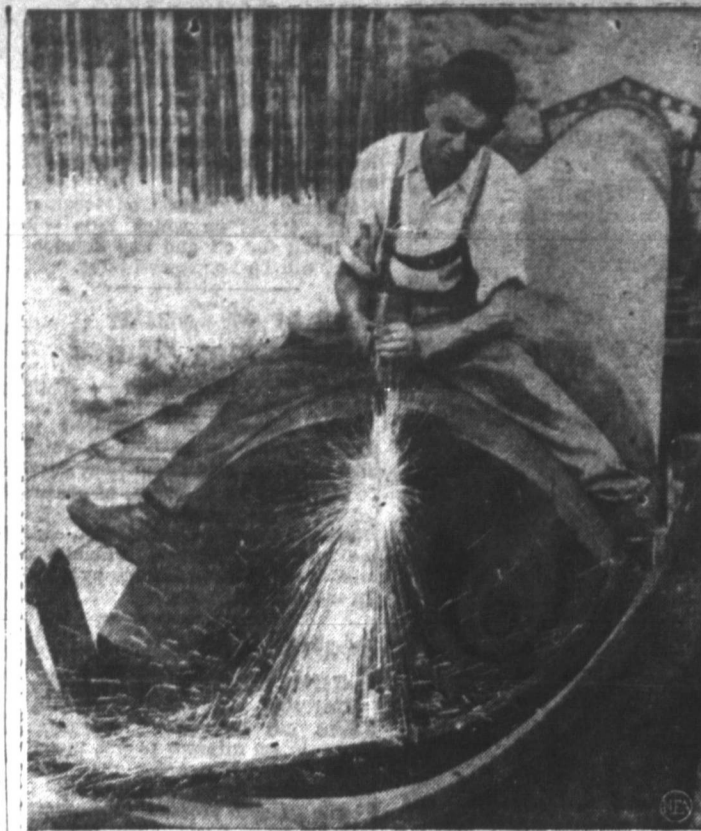
END OF A WAR-MAKER —Hitler's biggest long-range gun—used during the siege of Sevastopol in 1943—is dismantled on a railway track near Eschenbach, Germany. The 620-millimeter barrel, 100 feet long and weighing 136 tons, is being cut into four-foot chunks of metal. The modern Big Bertha was sold to a dismantling firm in Bavaria. (Photo by NEA-Acme staff correspondent Gerhard P. Seinig.)
