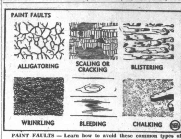
PAINT FAULTS — Learn how to avoid these common types of paint failure.
