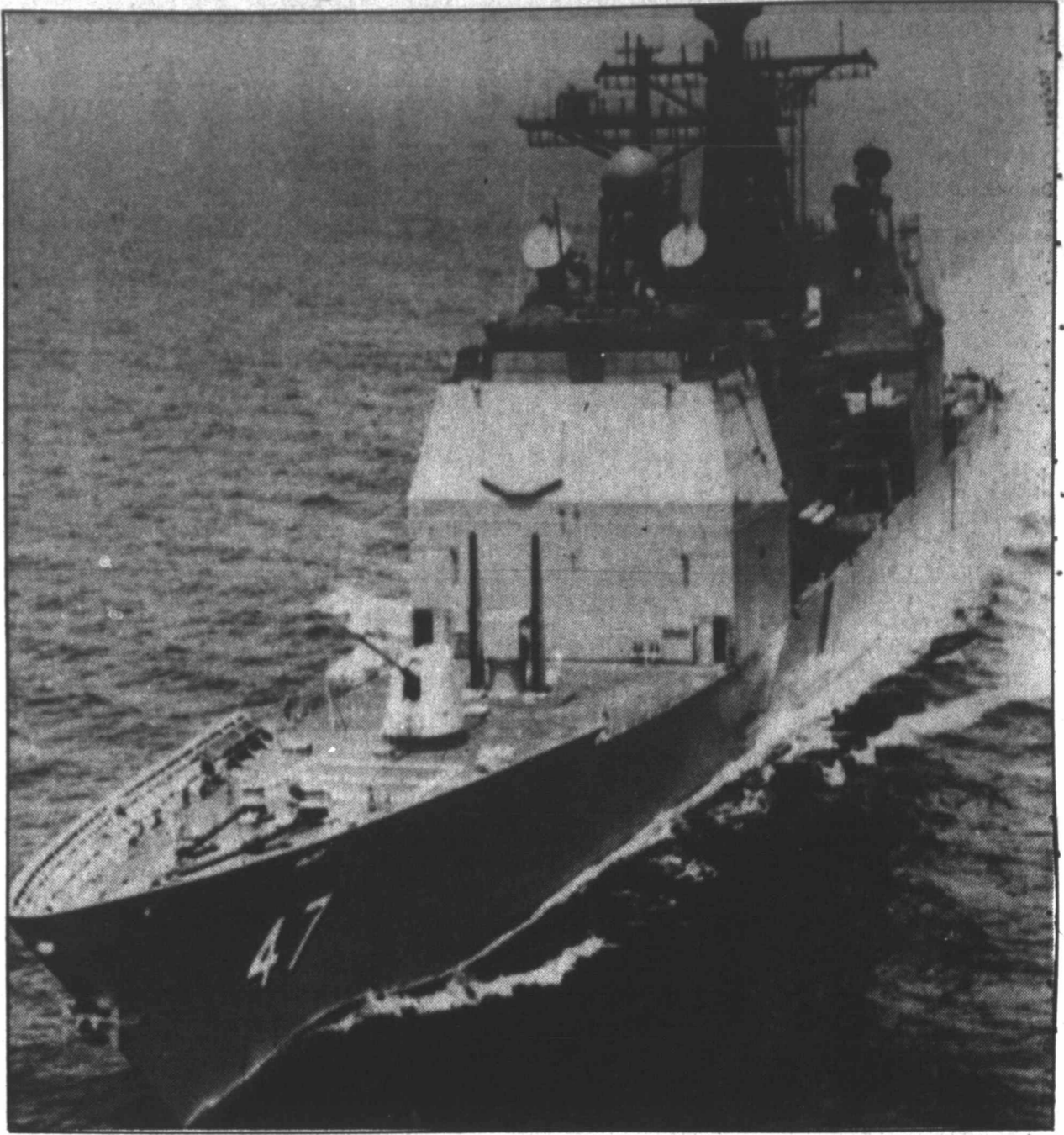
No one ever said it was perfect, but congressional investigators say the Ticonderoga, first of the Navy's Aegis Class guided missile cruisers, has real problems. It is top heavy, they said, and wants to roll over, and it is so heavy it cannot keep up with the aircraft carriers it was designed to protect. (AP Laserphoto)
