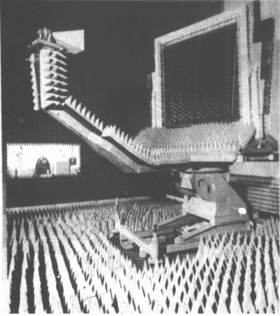
FUTURE RADAR. Grumman Aerospace is testing a section of a phased array antenna in its anechoic chamber with special walls to absorb the radar signals.
