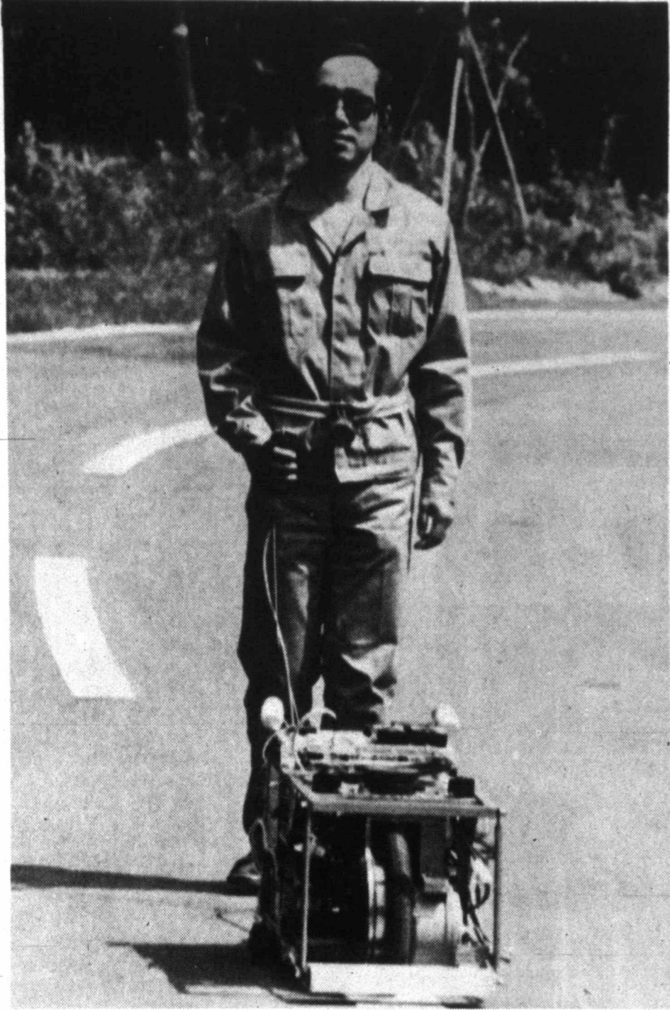
SEEING - EYE ROBOT. A researcher in Tokyo demonstrates MELDOG, a device built by scientists at the Ministry of International Trade and Industry to explore the concept of a mechanical seeing-eye dog for the blind. The developmental robot uses a variety of sensors to guide the blind "master" and warn of obstacles. The robot was demonstrated in Tokyo Sept. 15. (AP Laserphoto)
