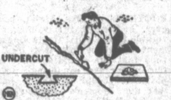
CLEAN, SHARP UNDERCUT IS NEEDED TO PROVIDE A KEY FOR THE NEW CONCRETE FILLING.
