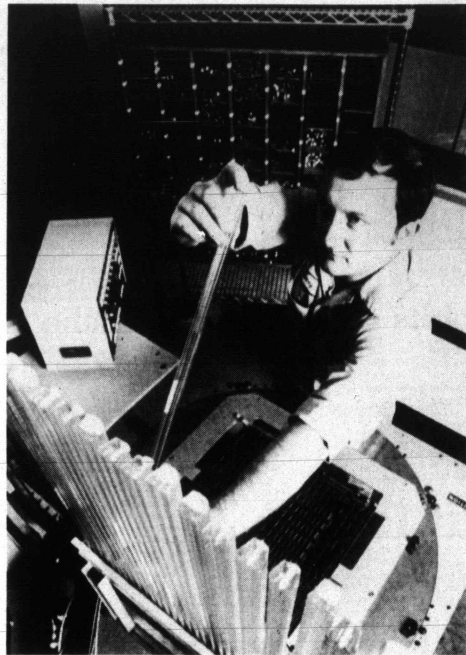
CHIP SHOT. A technician loads a high speed chip inserter at Computervision in Bedford, Mass. Chips are the nerve endings of the integrated circuit boards that
