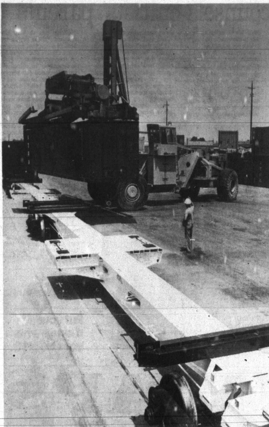
THE BARE BONES CONSTRUCTION utilized in Santa Fe Railway's new light-weight car for carrying freight containers is expected to produce a fuel savings of more than 15 percent compared with conventional equipment. Shipment of
