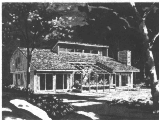
THIS REAR VIEW OF A passive solar energy house shows a sun garden and glazed walls facing south.
