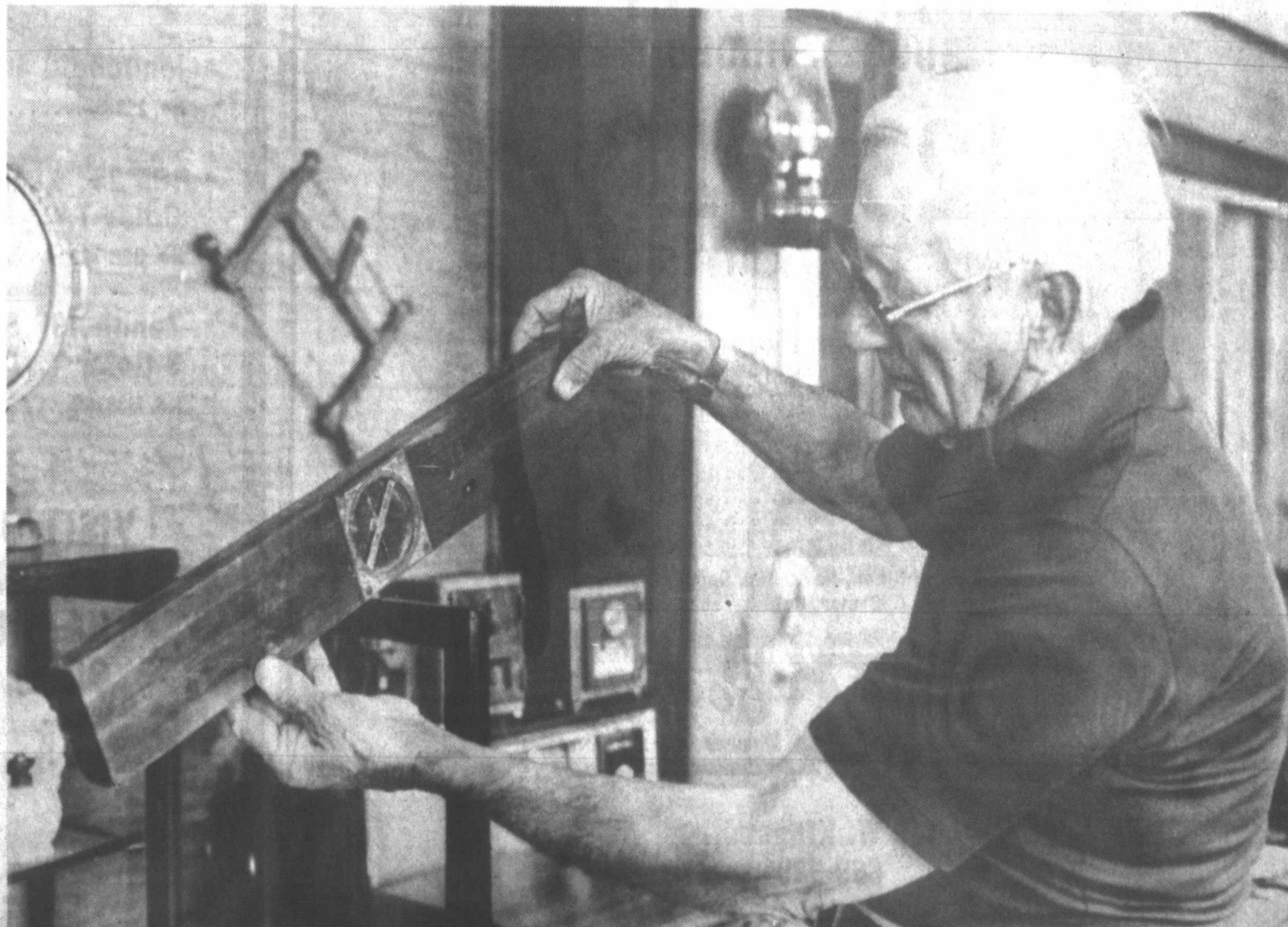
A LEVEL USED BY CRAFTSMEN YEARS AGO is now part of Philpott's collection of old tools. The collector demonstrates how housebuilders used the device to determine the pitch for setting rafters.
