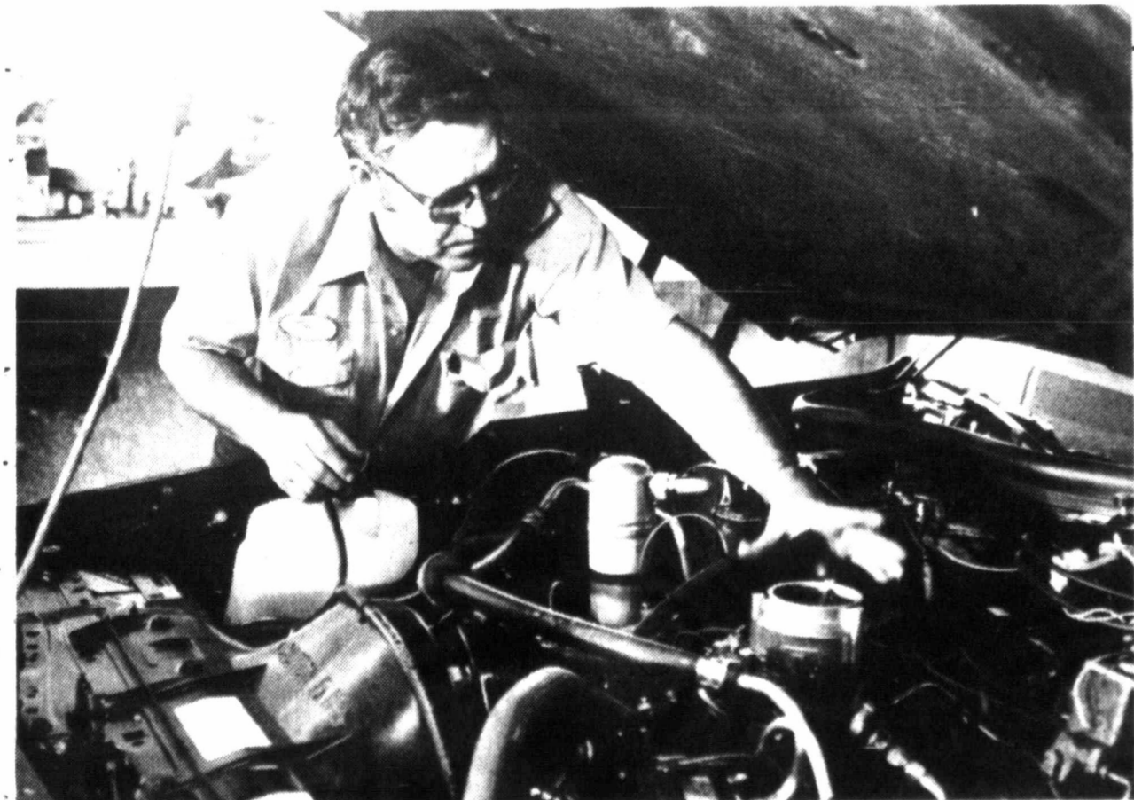
PROPANE-DRIVEN POLICE UNITS. Guy Cook of Pampa Oil Company installs a dual fuel system in one of two new Pampa Police Department units to be equipped with the system and a 28-gallon LPG tank, allowing the use of either gasoline or propane. Cook said the performance of the propane-driven units would equal that of gasoline-driven units, even though propane will only give 70 to 85 percent of the mileage of gasoline. The cost of propane is about half the price of the cost of gasoline, and a savings in fuel costs is expected. Pampa Oil Company won the low bid for the installation at approximately $600-700 per unit.
