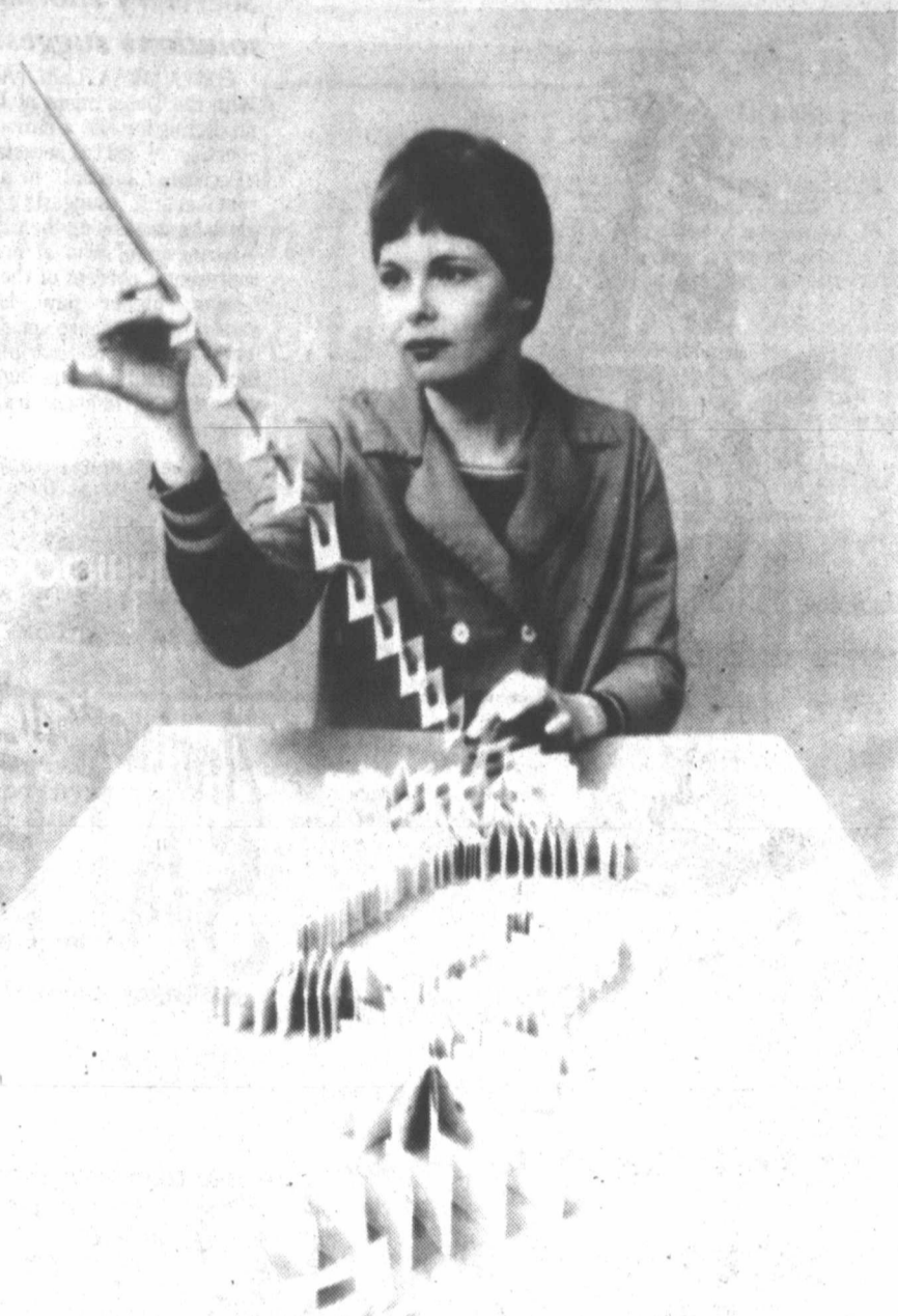
OIL SPILL DETECTION SYSTEMS made from laminated conductor cable is strung on rod by Carla Pidgeon of Emhart Corporation's Mailory Unit, prior to insertion into new oil spill detection system, in New York. The accordion-folded cable conducts the signals from sensing units, either on the surface or 100 feet underground reporting the presence of oil on ground water. The system is expected to reduce cost of oil cleanup.
