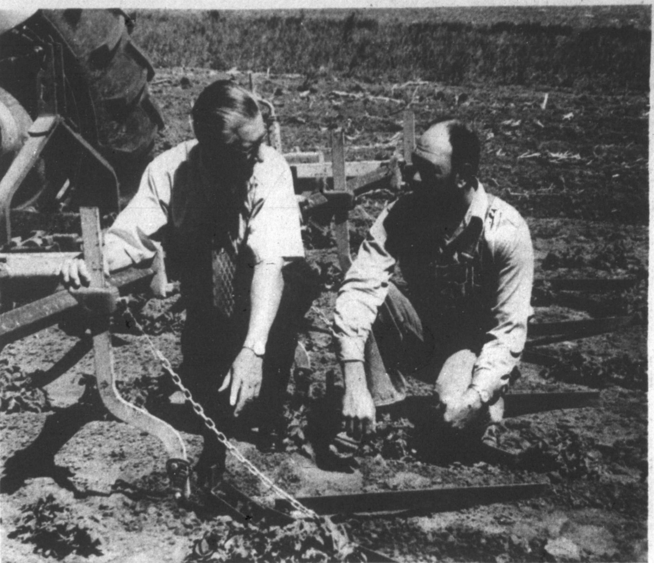
CULTIVATING SUPPLEMENT —Dr. A.W. Young, professor emeritus and retired chairman of the Department of Agronomy at Texas Tech University, left, instructs Tech nursery forman Donald Owen how his cultivator sweep supplement should be adjusted. The sweep supplement designed and developed by Dr. Young may be adjusted to push the soil loosened by the cultivator sweep toward the rows to the extent desired. The "chair" attached to the tool bar helps raise the sweep supplement for turning and may be used in adjusting the sweeps to the desired depth into the soil when cultivating. (Tech Pahto)
