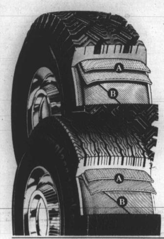
A Sturdy fiber glass double belting supports tread for good dig-in traction. (B) 2 tough polyester cord body plies provide resistance to tire-body damage.
