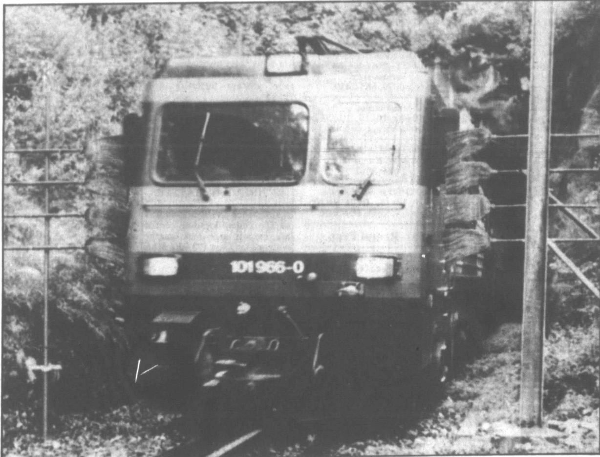
An engine of the single-track Swiss Bruenig Railway moves out of the Chaepeli tunnel, some 50 miles southwest of Lucerne, Switzerland. The train passes by poles with brooms fixed onto them that sweep against the side of the rail cars to warn passengers not to hang their heads out of the windows as the tunnel narrows. (AP photo/Keystone)
