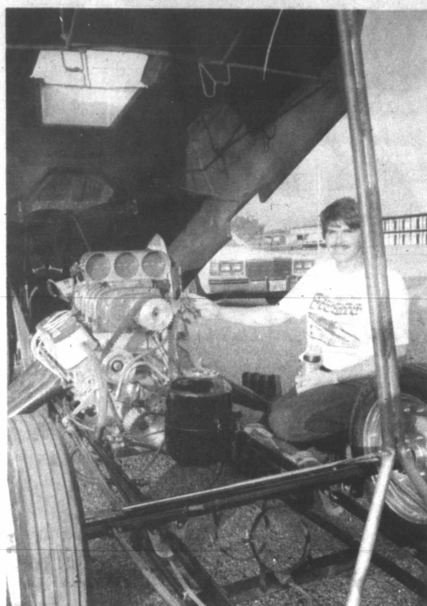
Chuck Kimball with his 1982 Plymouth Arrow funny car. It is a fiberglass body over a chrome-molybdenum chassis, with a 468 Chevy engine. An average run time for the car is 8:02 seconds in the quarter mile. That translates to 168 miles per hour.
