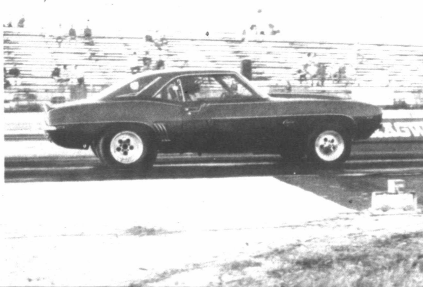
Johnson accelerates when the green light appears on the signal tree. Note the wrinkles in the rear tires. The air pressure in the tires is about 7 psi for better traction. The tire is screwed to the rim, otherwise the tire would spin off the wheel.
