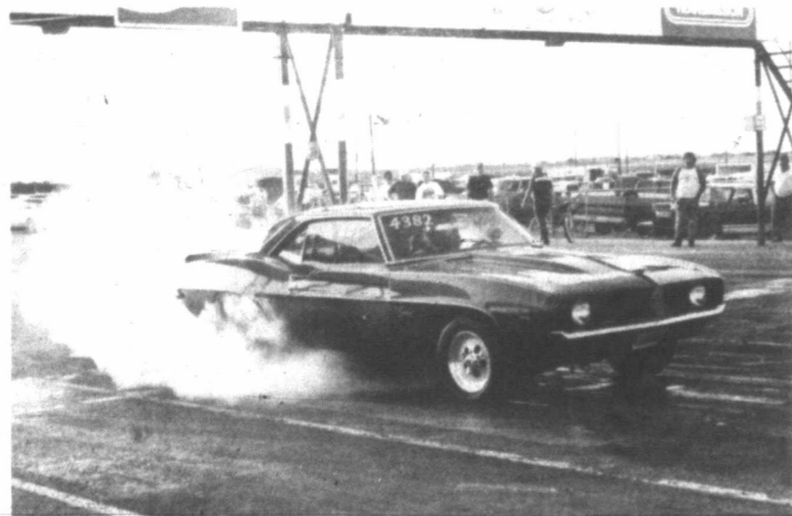
Johnson's 1969 Camaro in the "burn box", a pre-staging area. In the burn box, Johnson locks his front tire brakes, and spins the rear tires to heat and clean them. A cloud of acrid smoke and deafening noise is produced.
