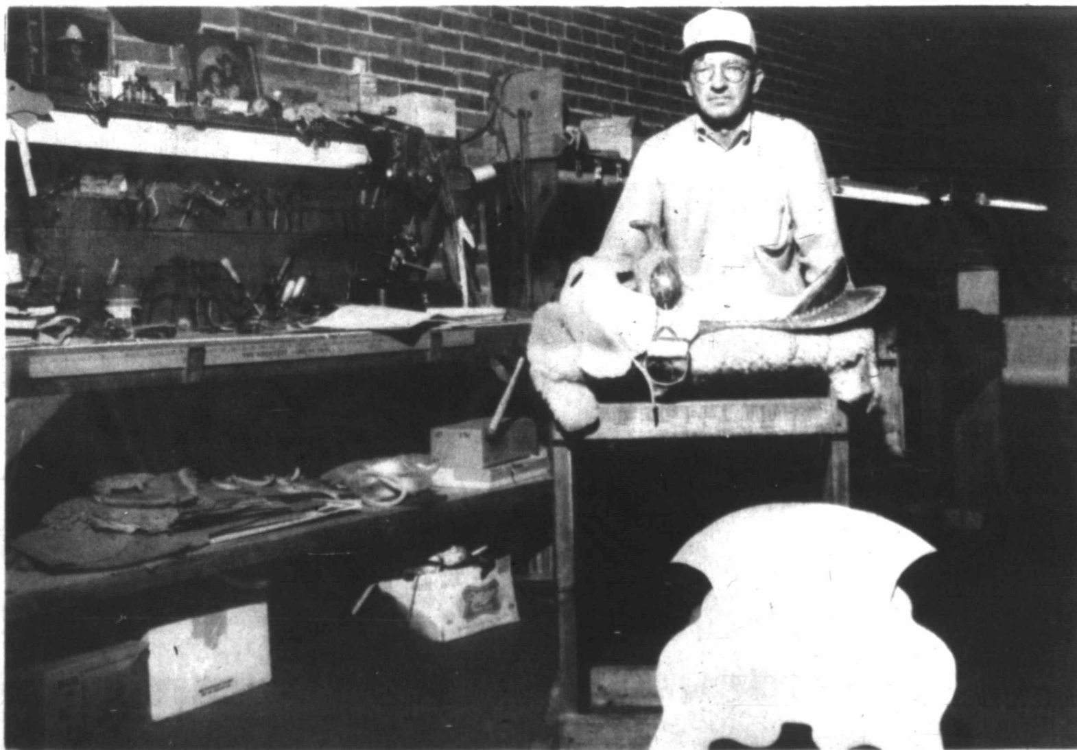
Another saddle under construction is ready to have the swells and seat covered. The riggings have been attached and the padding has been glued down. The glue used is wheat-based.
