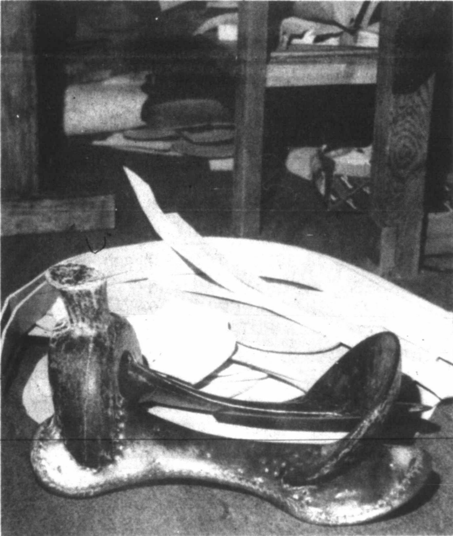
"Dave remembers a time when a saddle could be blocked out with two sides of leather. "Now you gotta be pretty careful to keep from getting into that third hide." Below, Nevada-style saddle tree with blocked out leather pieces is now ready for construction.
