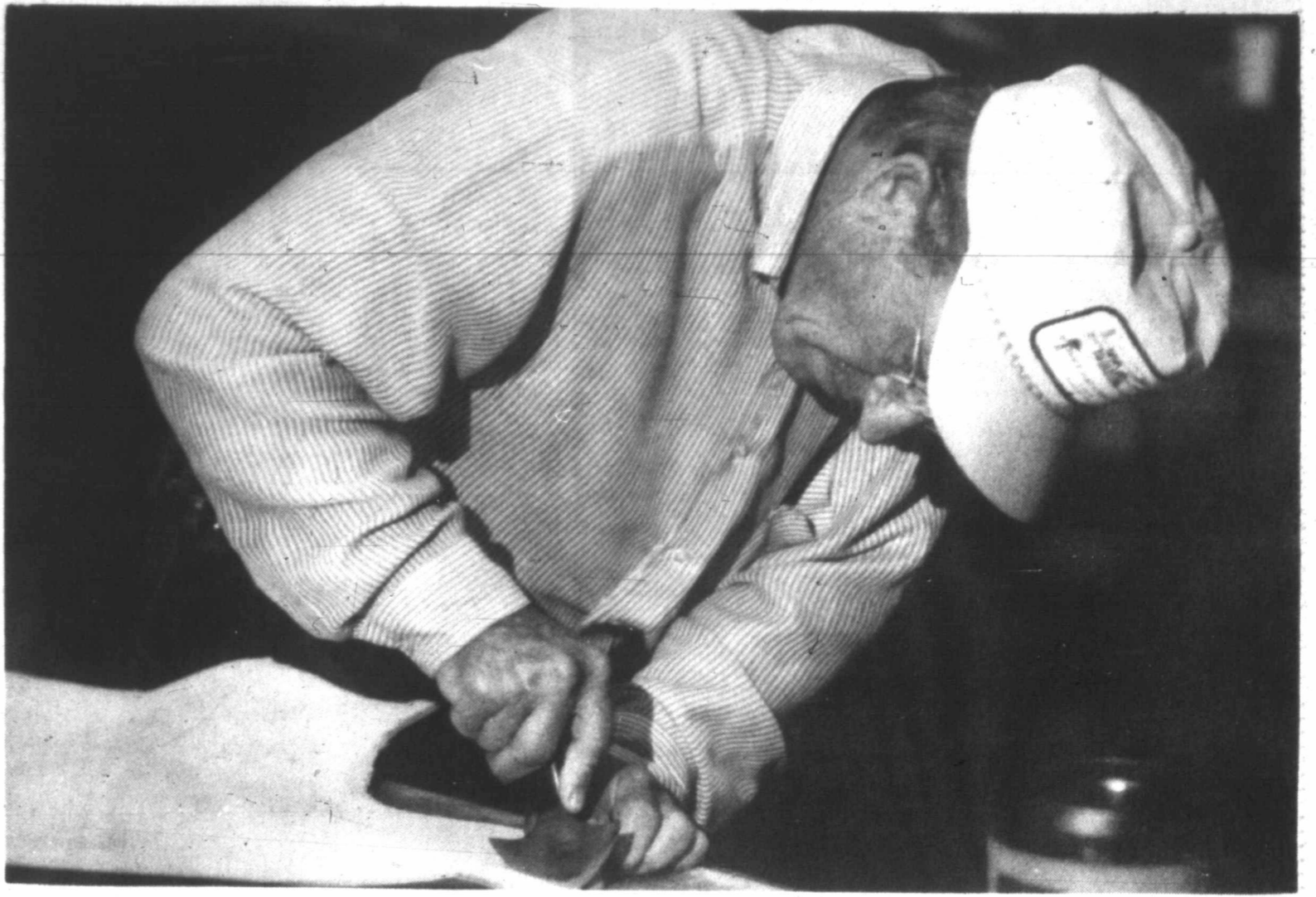
Dave Trimble, of the Rocking Chair Saddle Shop, uses a round knife (head knife) to block out patterns for a new saddle. Dave has been with the saddle shop for eight years.
