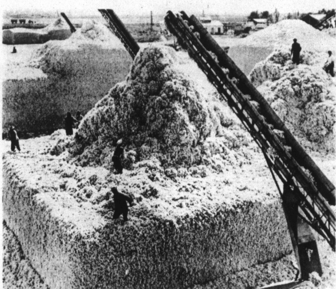
THOSE COTTON FIELDS BACK HOME — In Uzbekistan, USSR. This is a cotton depot in the Gagarin District of the Soviet Union. The angled conveyors carry the lint from transporting vehicles to rough piles atop the unusual squares of cotton where workers with forks level it in the manner of the square they are standing upon. Information is lacking on length of such storage — and on bales per acre. (NEA Photo)
