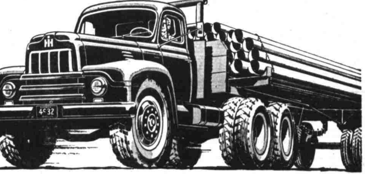
23 new 6-wheeler models. GVW ratings, 22,000 to 90,000 lbs. Choice of gasoline or LPO fuel systems. Diesel engines available for models with GVW ratings of 30,000 lbs. and over.
