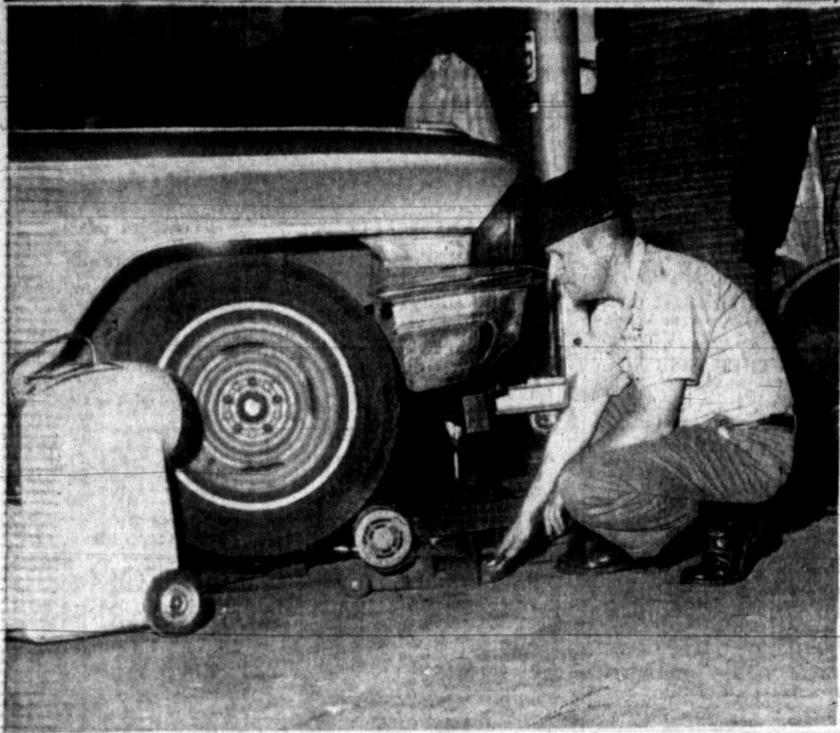
HE ADDS FUN TO YOUR MOTERING ... MILES TO YOUR TIRES Leymond Hall, owner-operator of Hall Tire Company, 700 W. Foster, MO 5-3755, trues tires (makes them perfectly round), balances them, aligns the front end, all to add pleasure to your driving, to give you extra wear. This is part of Hall's complete Tire Service. Here you get the best deal in town on new, first-line Security, Dayton, Mohawk Tires, and on quality Used Tires. Drive in. Let Hall check your tires while you select Seat Covers from his stock of covers to fit every make or model of car. Drive in for complete Tire Service.
