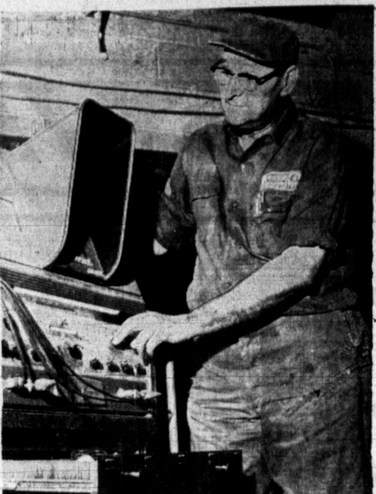
OLEN ANDERSON, owner and operator of Olen's Brake and Electric, 310 N. Ward, is shown with his Electronic Wheel Balancer which takes the guess work out of balancing your wheels. With this apparatus wheels can be checked up to speeds of 120 miles per hour. Olen also uses an Electronic Tune Up analyzer that shows the electrical condition of your engine.
