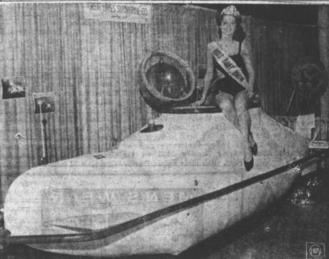
SUBMARINE BUILT FOR TWO is the newest item to intrigue boating enthusiasts. Shown at the Mid-America Boat Show in Cleveland, Ohio, the two-man undersea craft imported from West Germany operates to a depth of 115 feet, runs at five knots, and has a range of 12-20 miles or four hours before batteries operating its electric motor need recharging. Safety features: Oxygen supply, air scrubber to remove carbon dioxide, protection against diving too deep and an escape system if the sub cannot surface with the usual mechanism. Gracing the hull is Peggy Cheney of Campbell, Ohio, boat show queen.
