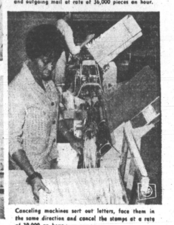
Canceling machines sort out letters, face them in the same direction and cancel the stamps at a rate of 30,000 an hour.
