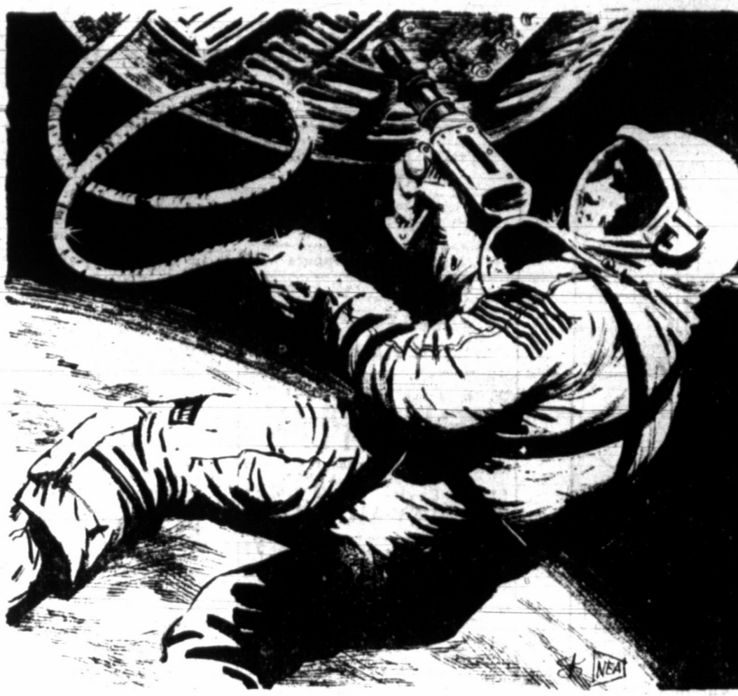
REPAIRMAN IN SPACE —Sketch above shows how astronaut David Scott will experiment with a new space power tool while "space-walking" out of the Gemini-8 capsule. He'll unbolt and rebolt a plate attached to the craft. The "minimum reaction" tool overcomes a physical law of action and reaction that prevents conventional hand tools from being used in an area of weightlessness.
